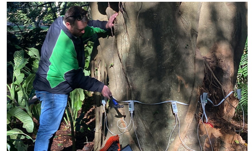
An arborist fixes the tomograph nodes in place, preparing to make an assessment on whether the tree has any cavities of structural weakness' inside.
