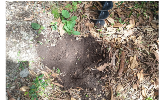
Preparations for the retrieval of soil samples along with a visual inspection of the soil layers.
