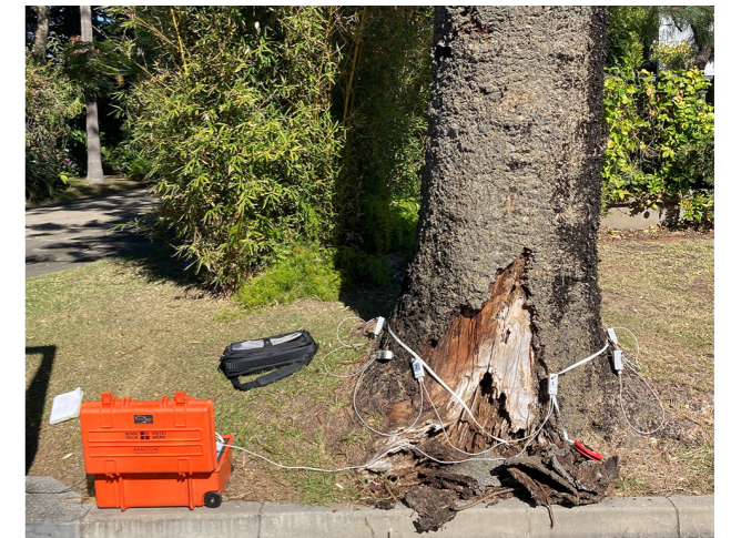
A sonic tomography setup and test as seen from the outside of the tree.
