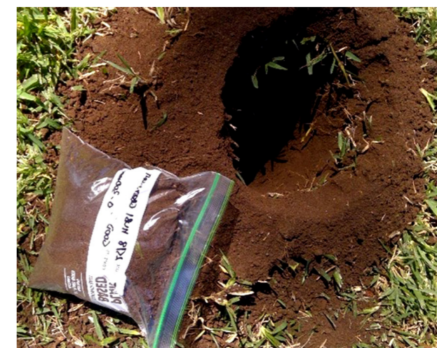
Vertical boring for investigation and soil sample retrieved for testing.
