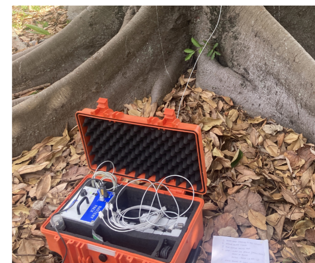
Tomograph testing being conducted to assess the tree's internal structure in a non-destructive manner.
