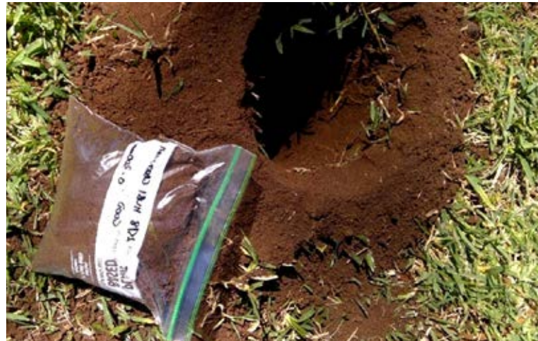
Vertical boring for investigation and soil sample retrieved for testing.
