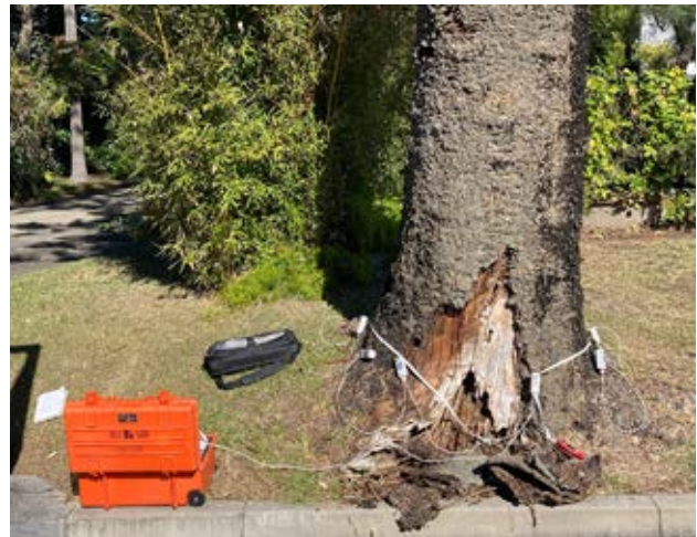
A sonic tomography setup and test as seen from the outside of the tree.
