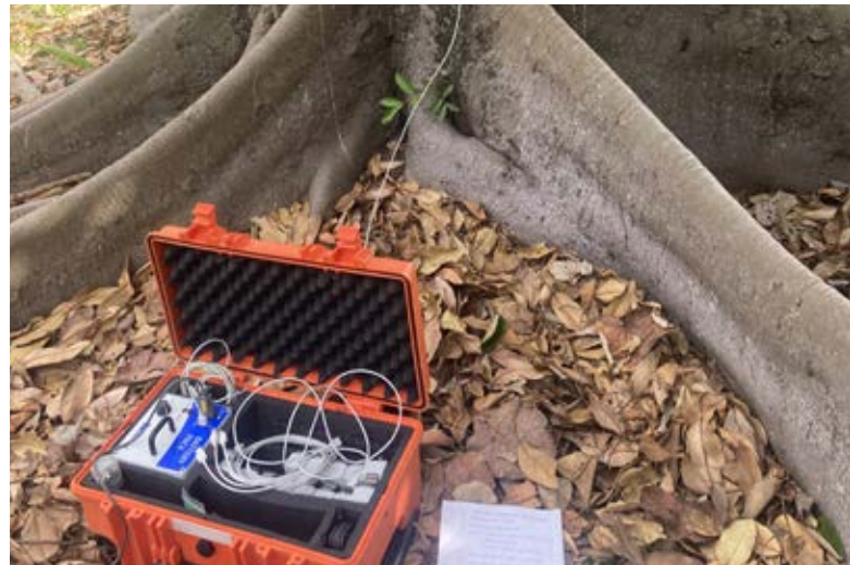
Tomograph testing being conducted to assess the tree's internal structure in a non destructive manner.
