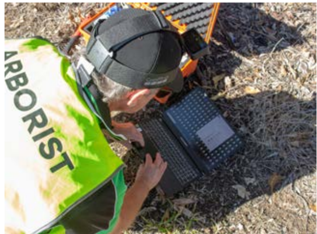
An arborist utilises the on-site tomographic scans to make an educated deduction of the condition of the tree.
